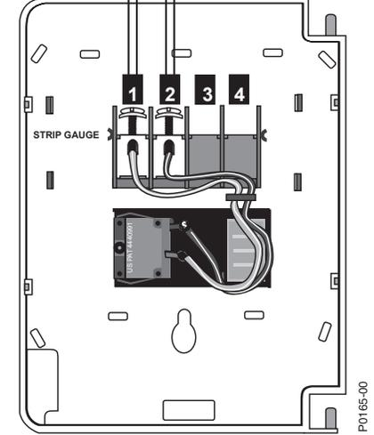
\*Mount End of line resistor on last unit.
