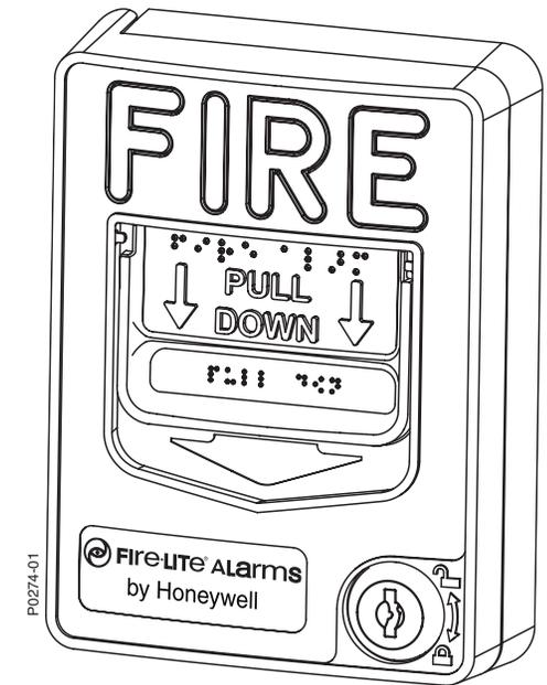
**CAUTION!** Do not detach the door of the pull station during installation. The door of the pull station cannot be reattached to the backplate after the backplate has already been installed onto an electrical box.
