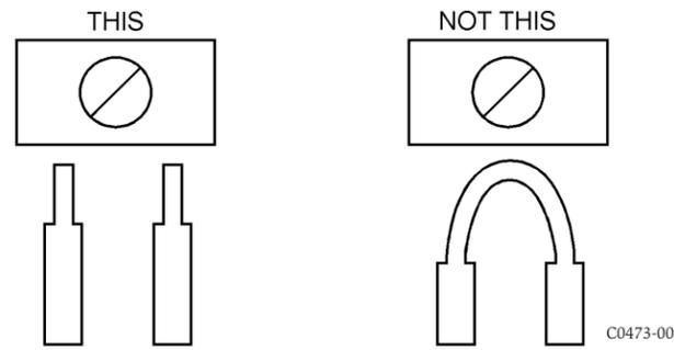
DO NOT loop the wire under the clamping plate.
