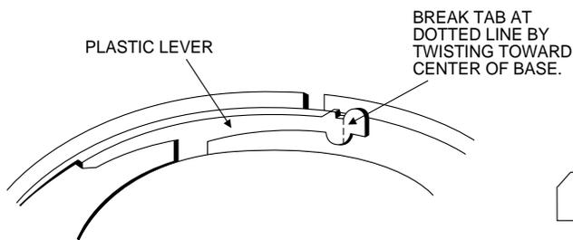
**Figure 3B. Removing the detector head from the base:**
