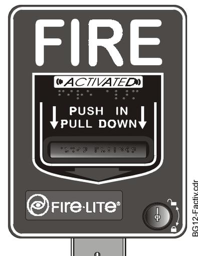
The pull station includes one Double Pole, Single Throw (DPST) Normally Open (N/O) switch which closes upon activation of the pull station.
