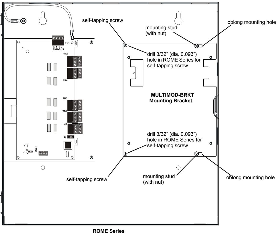
7. Install the supplied module insulating pad on the MULTIMOD-BRKT bracket by aligning the four outer holes with the four standoffs on the bracket and pressing the pad onto the standoffs and flat against the bracket as illustrated below.
