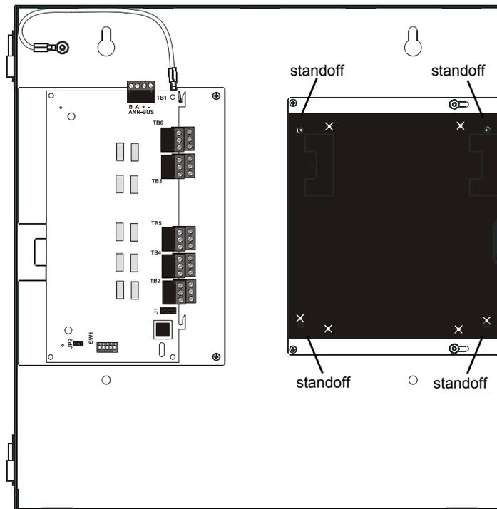
8. Install the addressable Multi-Module on the MULTIMOD-BRKT mounting bracket by positioning the four module mounting holes over the four standoffs on the mounting bracket.
