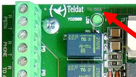
**Figure 5. Board identification details**
