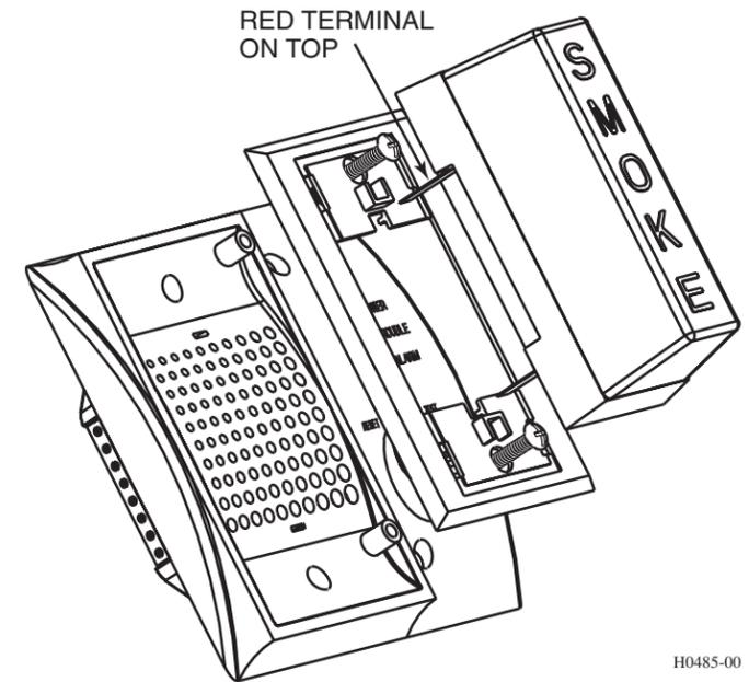
The PS24LO strobe will be mounted on top of the sounder, on the left-hand side of the SSK451. Place one mounting spacer between the SSK451 and the strobe adapter plate at each screw attachment location. Attach the adapter plate, spacer and SSK451 to the left-hand side of the double-gang electrical outlet box with two mounting screws.
